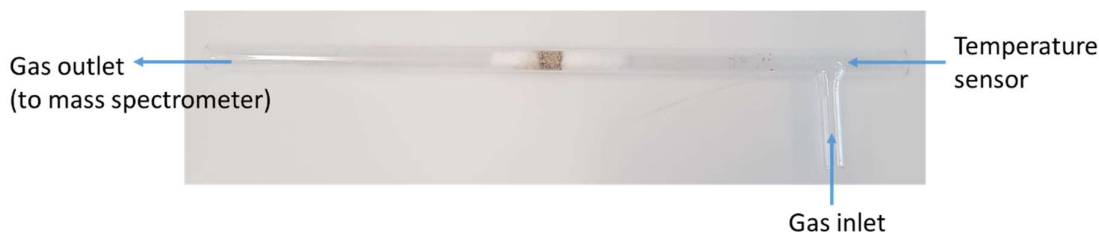
Figure 2. Plug flow reactor to study catalysts in powder form.
